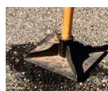
2. Compact fill mix. The material should be compacted so that the surface of the fill is level or slightly above the surface of the roadway.
